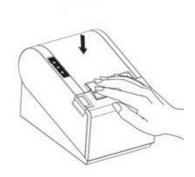
(4) Use the cutter of printer to tear off the extra paper
