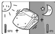
Places with high temperature drops or condensation corrosion
