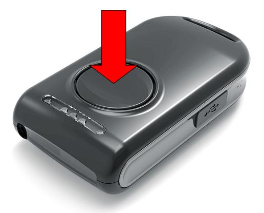
You will head two beep sounds. Release the button. Now the scanner is in pairing mode and can be browsed from the PDA, smart phone or a PC.
